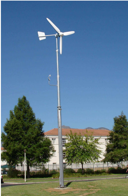
Figure 2: 3 kW wind generator being tested in front of the engineering building
