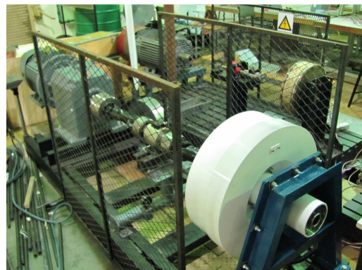
Figure 1: Antarctic 20 kW direct drive PM wind generator under test in the EMLab laboratory.
